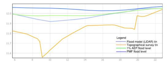
Figure 7 – Comparison of Tins and Flood Levels ("Sydney Light Rail Flood GIS Model (Model Version 107)" by Transport for NSW, June 2017)
