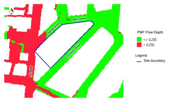
Figure 15 – Floodplain classification according to Peak Flood Depth Probable Maximum Flood (PMF) ("*Sydney Light Rail Flood GIS Model* (Model Version 107)" by Transport for NSW, June 2017)
