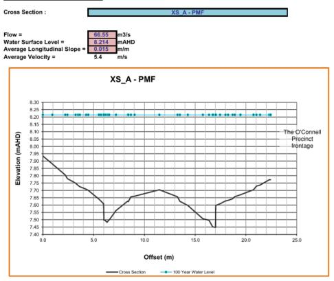
Figure 11 – Cross Section A Overland Flow Assessment, Peak PMF Flow
