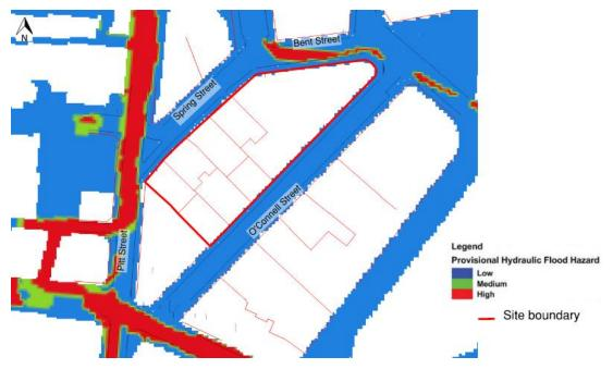
Figure 13 – Provisional Hydraulic Hazard 1% AEP (100 yr ARI) ("City Area Catchment Flood Study", BMT, October 2014)
