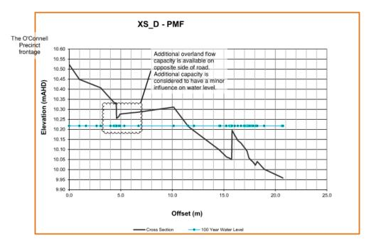
Figure 17 – Cross Section D Overland Flow Assessment, Peak PMF Flow
