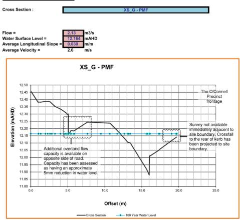
Figure 12 – Cross Section G Overland Flow Assessment, Peak PMF Flow
